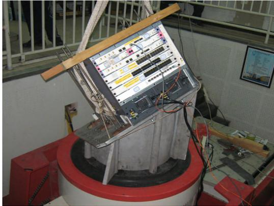
Network blades on skewed ESS system at Huawei
