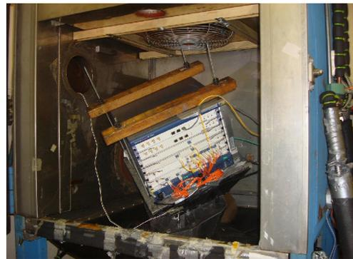
*Network Blade on Quanta's ED Shaker/Chamber with Skewed Fixture*
