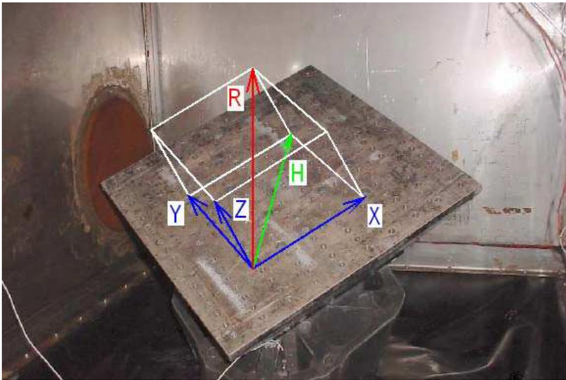
Quanta Laboratories' Skewed Fixture with Electro-Dynamic Shaker System
