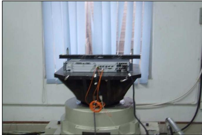
Single Axis ED Shaker at Huawei
